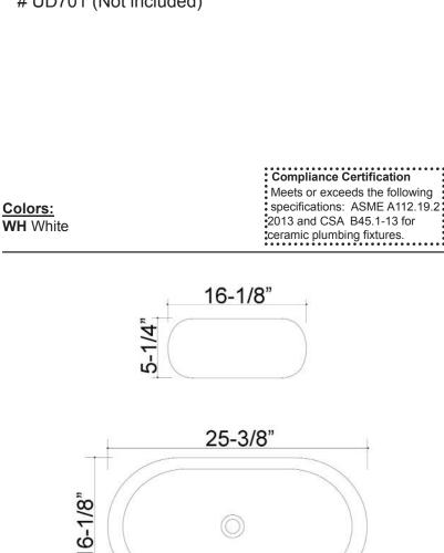
Dimensions of fixture are nominal and may vary within the range of tolerances established by AMSE Standard A112.19.2.2013 Dimensions and specifications subject to change without notice.
